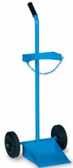
● MG420 Carrello portabombole. Ruote Ø 200 mm Portata 200 kg. bombola Ø 250 lt.40 Trolley for tanks. Wheels ø 200 mm Capacity 200 kg. Can ø 250 lt 40 | Diable porte bouteilles Roues diam. 200 mm. Charge 200 kg. Bouteille diam. 250 mm lt.40 l. 250 / p. 380 / h. 1150
